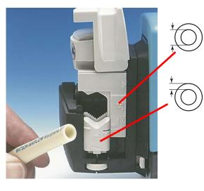
Set the tube clamps to the correct tube size. The track must be fully open. Align the scale on both sides of the pumphead.
